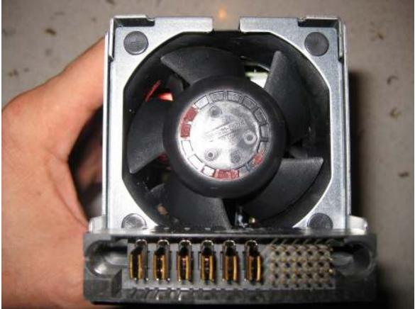
Left 3 large contacts - +12V, Right 3 Large contacts - common (and case) Pin contacts - A is bottom row, D is top row, pin 6 is to the far right.
